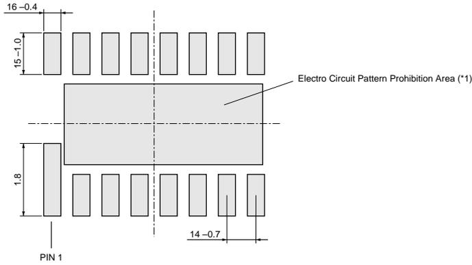
The GND Pattern for Electric Shield. (2<sup>nd</sup> layer) (\*2)
