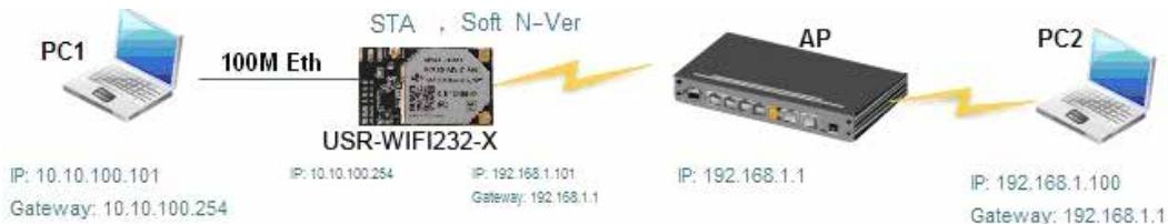
**Figure 20 USR-WIFI232-X Ethernet Interface Networking (As STA, N-Ver)**
