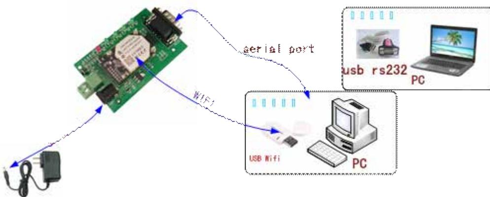
**Figure 30 Connection diagram**
