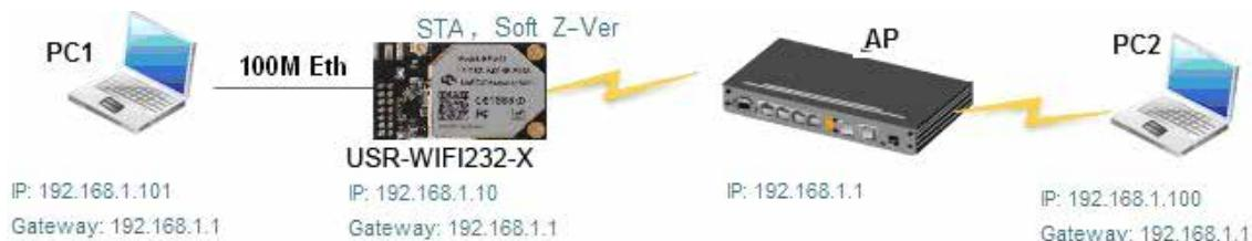
**Figure 21 USR-WIFI232-X Ethernet Interface Networking (As STA, Z-Ver)**
