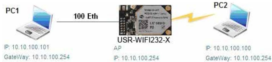
**Figure 19 USR-WIFI232-X Ethernet Interface Networking (As AP)**
