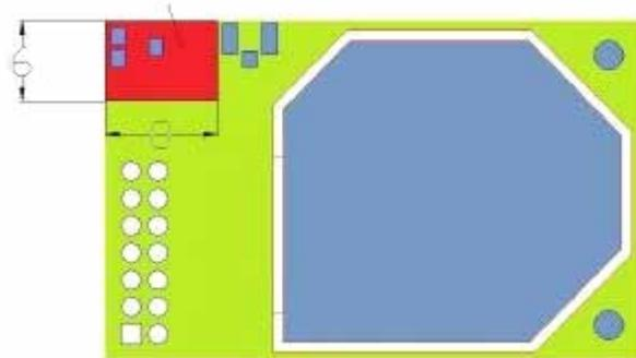
**Figure 4 USR-WIFI232-X Chip Antenna Keep Out Region**
