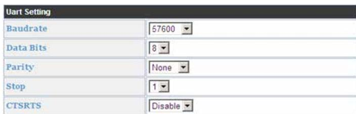
**Figure 38 USR-WIFI232-X Default UART Port Parameters**
