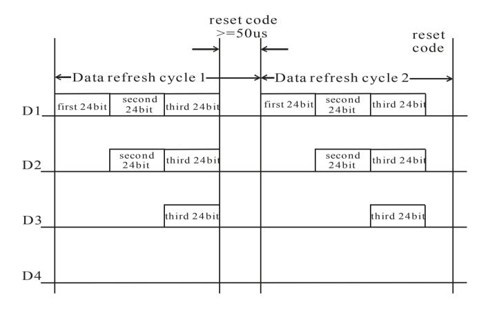
Note: The data of D1 is send by MCU, and D2, D3, D4 through pixel internal reshaping amplification to transmit.
