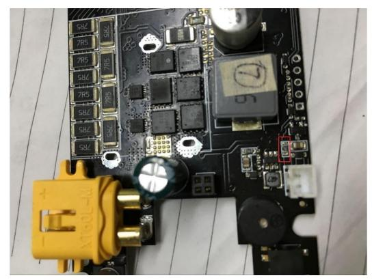
2: short circuit by soldering at same spot (bridge)
