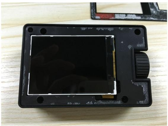
$\Box$ , Gently open the acrylic screen, note the cable interface in red circle, gently remove the it
