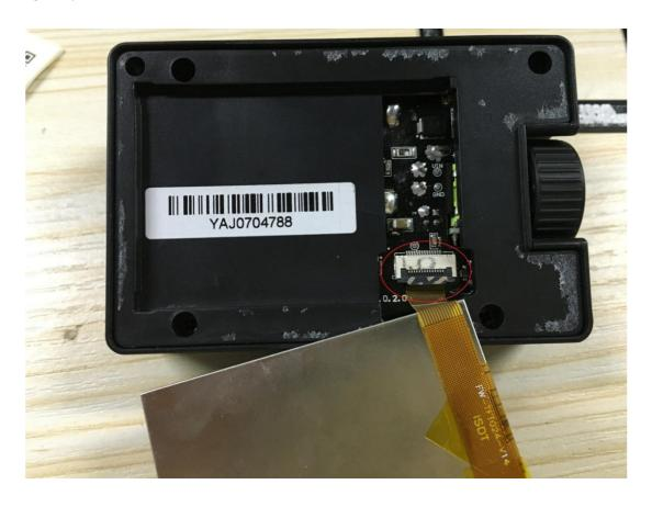
$\equiv$ . Note the location of the four screws in the figure below, remove the screw and the cover
