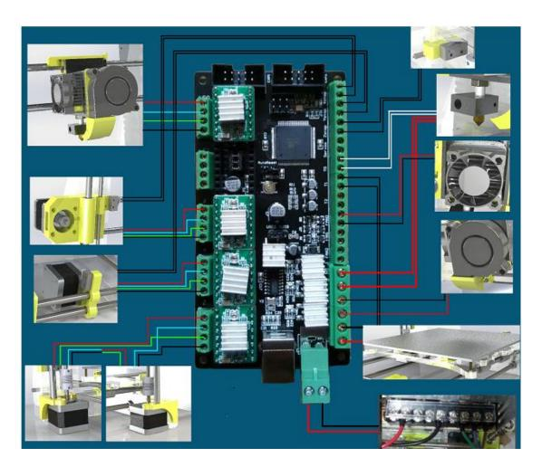
This is the wiring of power box: connect the red to V+, black to V-, and the power line with a plug is on the right end.
