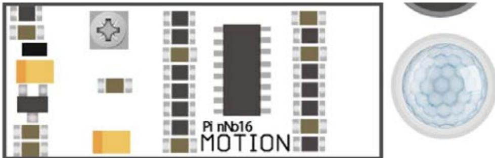
The motion sensor is one of the most useful and often used sensors out there. As you've seen in our kick-starter video, we used the motion sensor to detect a thief coming in and trying to steal our CrowPi ... by detecting their motion using infra-red light, we were able turn on a buzzer alarm and make the thief run away!
