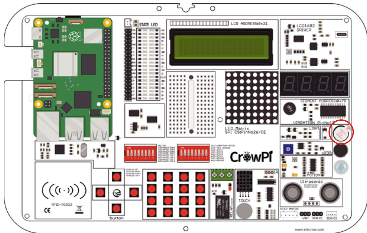
The first time you use your Raspberry Pi, the Buzzer sensor might be sealed with a protective sticker.
