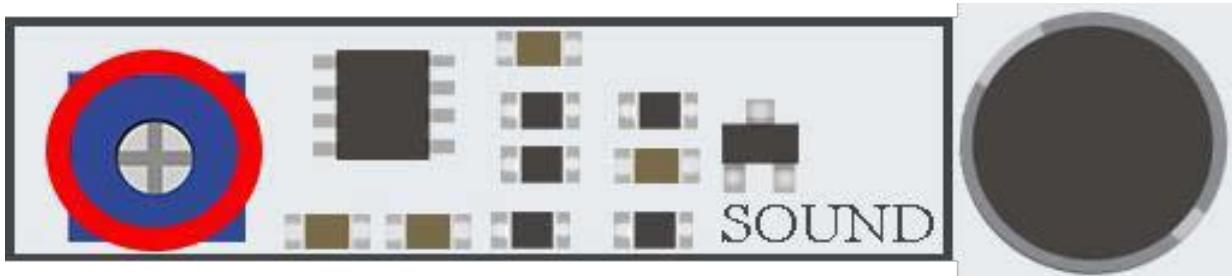
We'll need to turn the little blue square that is circled with a red oval in the picture to either left or right in order to control its sensitivity.
