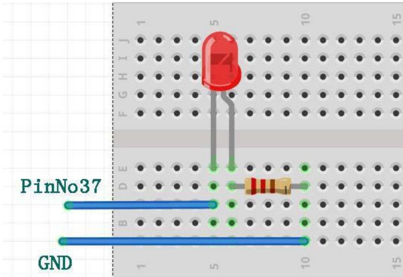
You can refer to this picture to make your circuit on the breadboard. Don't forget that PinNo37 is located on the SERVO1 Interface GPIO port. The GND is located on the SERVO1 Interface as well on the GND port.
