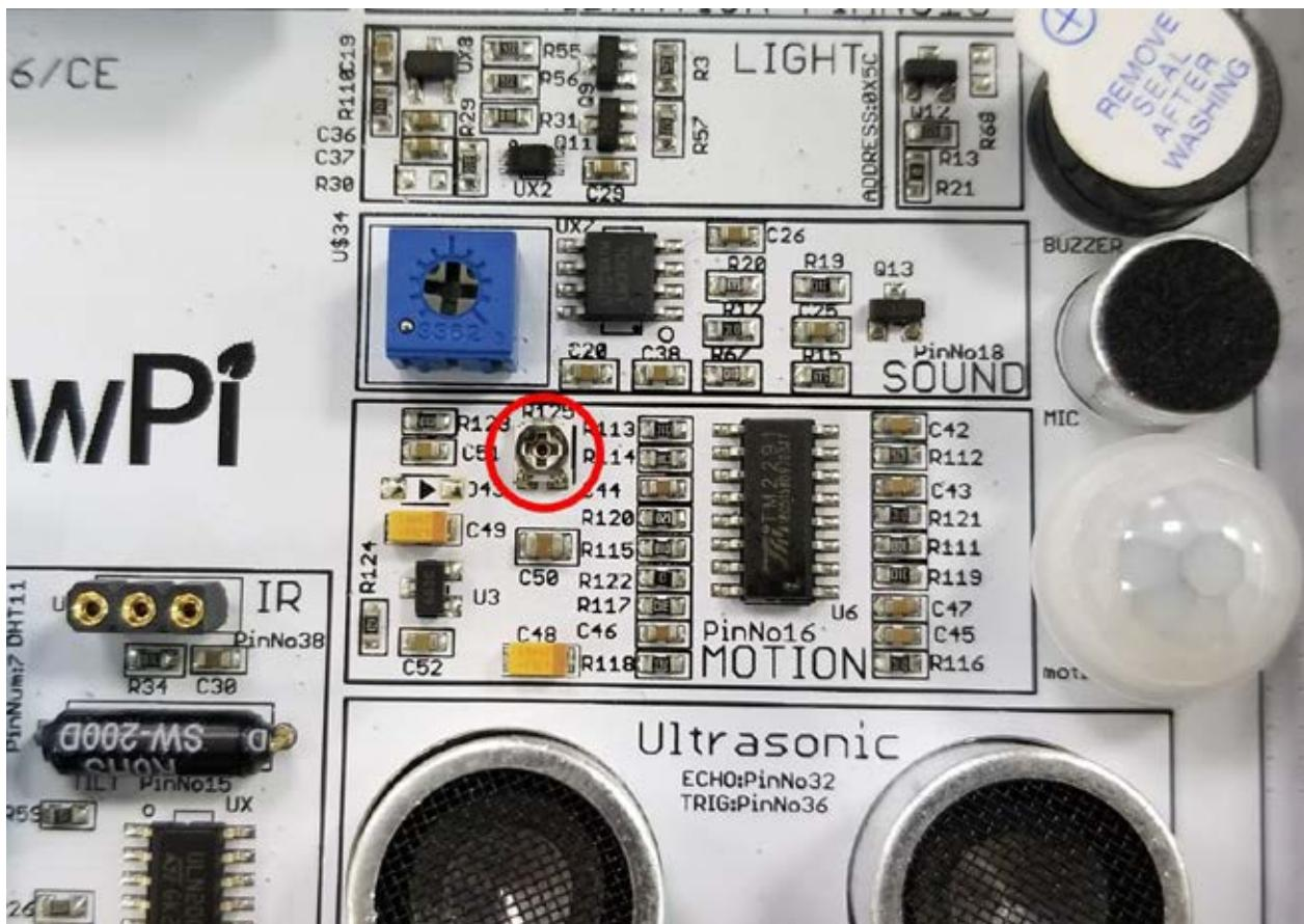
By using a standard Philips flat head screwdriver, rotate the screw to the right or to the left when running the motion example script in order to find a suitable distance for the motion sensor.
