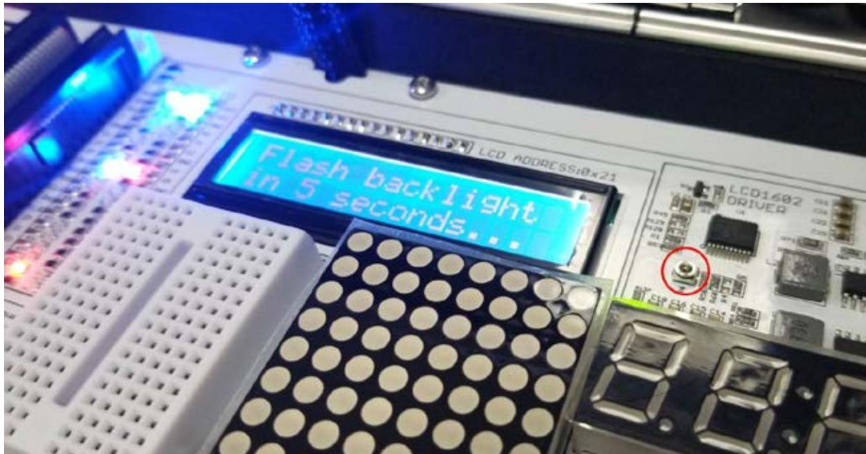
By using a standard Philips screwdriver, rotate the screw to the right or to the left when running the LCD example script in order to find the suitable brightness for you.
