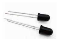
The flame sensor can be used to detect fire or other wavelength at 760 nm ~ 1100 nm light. In the fire-fighting robot game, the flame plays an important role in the probe, which can be used as the robot's eyes to find fire source or football. It can make use of fire-fighting robots, soccer robots.
