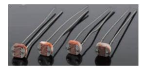
As the resistance of the sensor varies depending on the amount of light it is exposed to, the output voltage changes with the light intensity. It can be used to trigger other modules.
