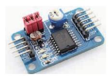
The PCF8591 module an 8-bit A/D Converter & D/A Converter PCF8591 with four analog inputs, one analog output and a serial I2C-bus interface.
