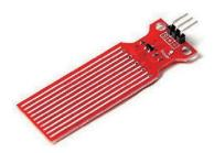
This is a water level measurement experiment, it is relatively simple to achieve, only need to read the value of the analog port(A0 or others), and then converted to a percentage.
