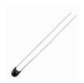
The resistance of a thermistor increases when the ambient temperature decreases, so the RPI can detects the voltage and thus to caculate the current temperature. The detection range of this sensor is between -40 to 125 degrees Celsius with an accuracy of  $\pm 1.5^{\circ}$ C.
