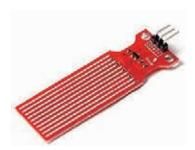
This is a water level measurement experiment, it is relatively simple to achieve, only need to read the value of the analog port(A0 or others), and then converted to a percentage.
