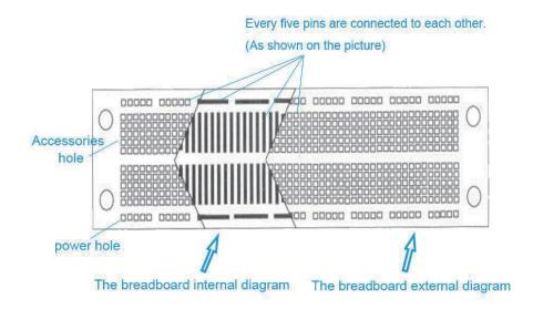
All the tie points (indicated in the picture) of the different colors are connected together.
