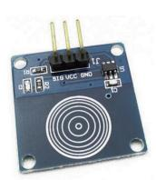
This is a touch sensor to control the LED lamp experiment, it can control each LED light, but also can achieve the effect of breathing light.
