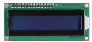
This is an experiment on how to use LCD1602 with IIC, the next lesson will do a temperature and humidity monitoring experiment.
