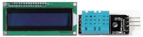
This is a more complex experiment, it can realize the monitoring of indoor temperature and humidity, and in the LCD above display value.
