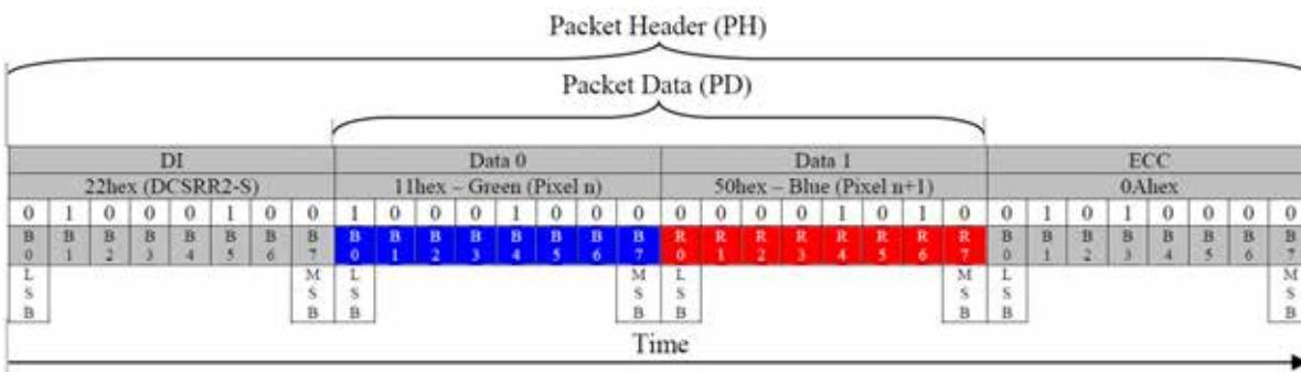
**Figure 100: Blue and Red Sub-pixels Response (DCSRR2-S) – Example 7**
