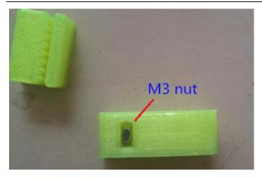
Tighten the belt with M3x30 screw
