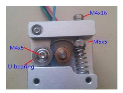
Fix to the U-chassis following the picture below, put the pipe through the hole of baseboard to the M6 hole of the Extruder. Pay attention to the direction of the pipe! Don't pull out the plastic pipe! About 15mm outside the pipe and install the heating piece and nozzle lastly.
