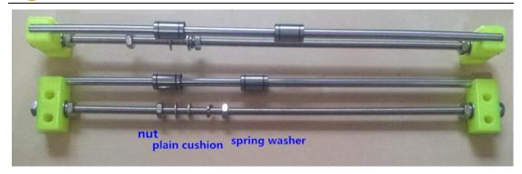
Take out the second assembled component, install the front- end of printer as follow
