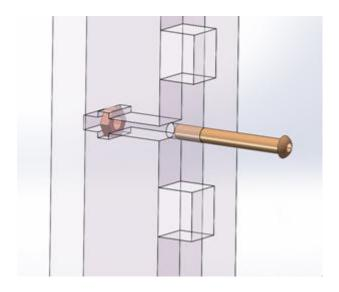
Use M3\*25 screw to connect the Acrylic framework. Pay attention to the red circling part. The part with three holes is on the right side for fixing the power supply and fixed hole of other side is different due to the different control panel.
