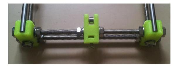
Take out the assembled motor part of Y-axis at the first step and assemble the rear-end of the frame following the picture. The distance of both sides as below should be the same.
