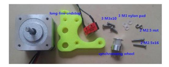
Assemble all the components as below, separate the blue circling part between motor and motor frame with a nylon pad.
