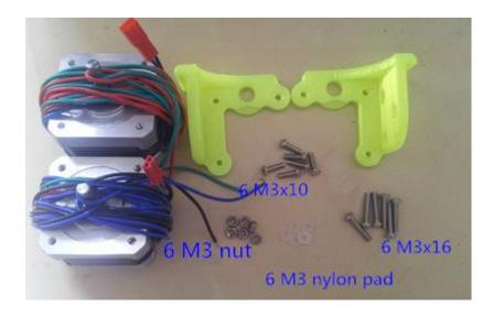
Assemble the components as the following picture and fix the back side with M3 nut
