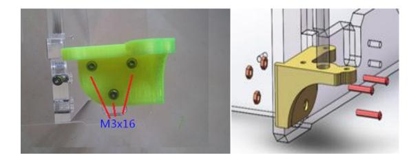
Separate the motor and the plastic part with a nylon pad Make your making more easy!
