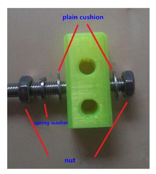
After assembling as below, reserve 2 nuts, 2 plain cushion and 1 spring washer on the threaded rod.
