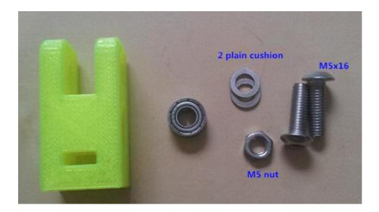
After assembling, don't screw up the screw through axle bearing and leave enough space for the axle bearing to rotate.
