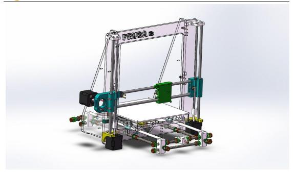
Make the Triangular side panel and threaded rod fixed as below and note that the threaded rod should stuck into the inner side of the groove of the Acrylic framework.
