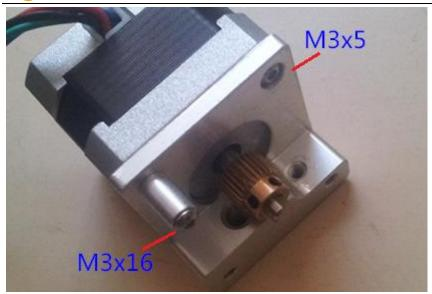
Install the toothed gear, bearing, and the spring washer as follow
