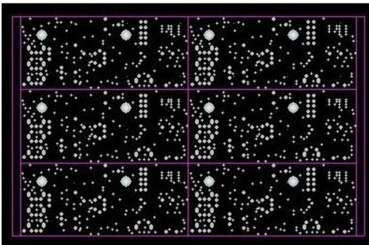
8. The minimum distance between the hole is 10mil to avoid the hole don't have copper.
