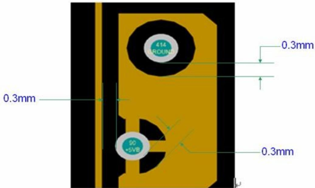
5. For grid copper, The minimum space and wire size is 10mil. A Whole copper is recommended to avoid some break problem.
