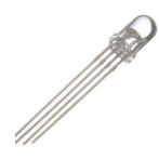
In this lesson, you will learn how to use a RGB (Red Green Blue) LED with an Arduino. You will use the analogWrite function of Arduino to control the color of the LED.
