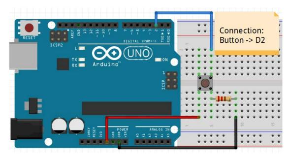
Connect three wires to the board. The first two, red and black, connect to the two long vertical rows on the side of the breadboard to provide access to the 5 volt supply and ground. The third wire goes from digital pin 2 to one leg of the pushbutton. That same leg of the button connects through a pull-down resistor (here 10K ohm) to ground. The other leg of the button connects to the 5 volt supply.
