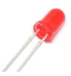
The LED is designed for the beginners of Arduino. Blinking LED experiment is quite simple and it is the best choice to help you learn I/O pins. On this lesson, we are going to connect an LED to one of the digital pins.
