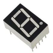
The 7-segment display, also written as "seven segment display", consists of seven LEDs (hence its name) arranged in a rectangular fashion as shown. Each of the seven LEDs is called a segment because when illuminated the segment forms part of a numerical digit (both Decimal and Hex) to be displayed.
