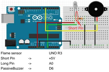
Note: The short pin of the Flame sensor is connected to +5v.
