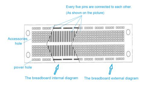
All the tie points (indicated in the picture) of the different colors are connected together.
