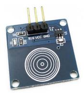
This is a touch sensor to control the LED lamp experiment, it can control each LED light, but also can achieve the effect of breathing light.
