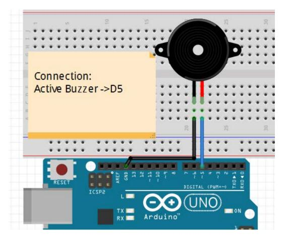
Note: The longest active buzzer of the pin is connected to the digital signal port 5 (D5).
