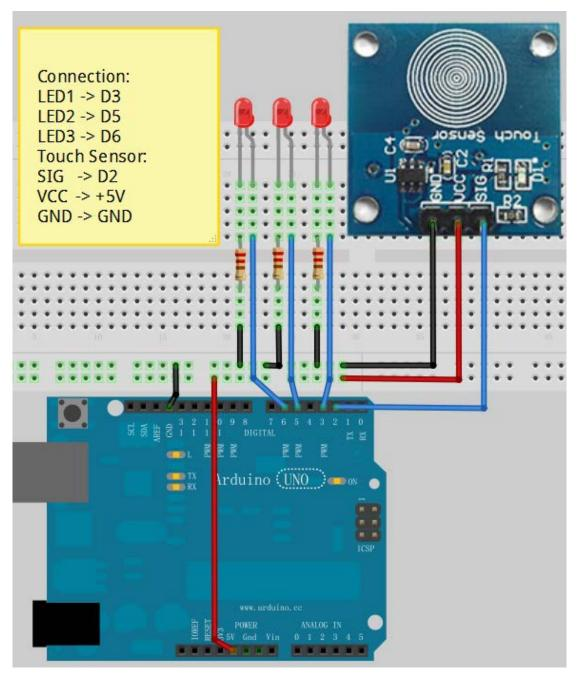
Note: The longest LED of the pin is connected to the digital signal port.
