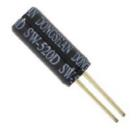
This tilt switch can easily be used to detect orientation. Inside the can is a ball that make contact with the pins when the case is upright. Tilt the case over and the balls don't touch, thus not making a connection.
