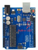
Button switches, familiar to most of us, are a switch value (digital value) component. When it's pressed, the circuit is in closed (conducting) state. This example turns on the built-in LED on pin 13 when you press the button.
