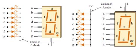
In general, common anode displays are more popular as many logic circuits can sink more current than they can source. Also note that a common cathode display is not a direct replacement in a circuit for a common anode display and vice versa, as it is the same as connecting the LEDs in reverse, and hence light emission will not take place.
