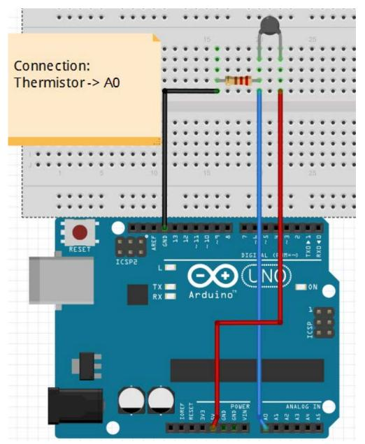
Note: Thermistor `s pin does not distinguish between positive and negative poles.
