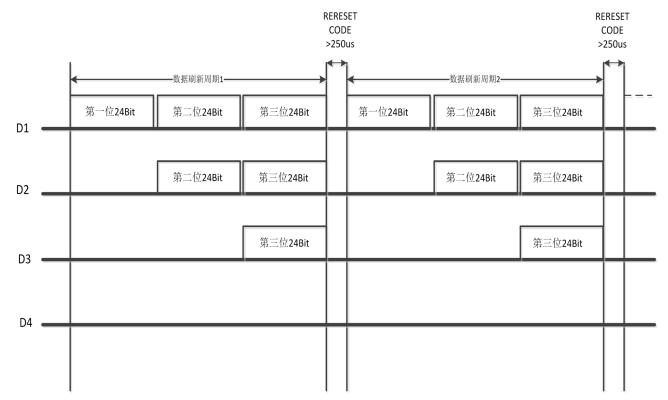
Note: D1 is the data from MCU, and D2, D3, D4 are from Cascade Circuits.
