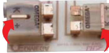
† A mounting bracket is supplied with each connector and must be used to securely mount the connector to the PC board.
