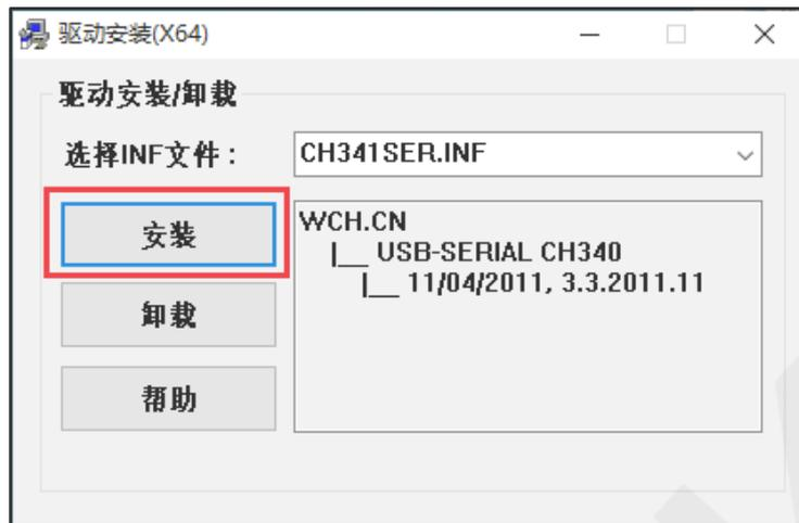
Figure 5.1 Installing the CH340C driver
