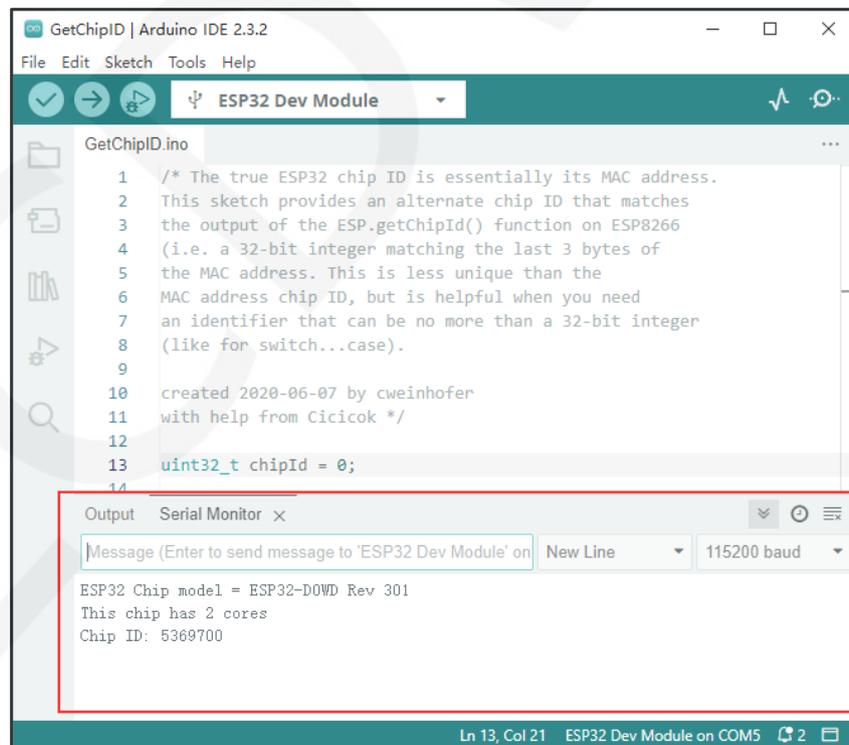
Figure 5.9 Serial port output of ESP32 program
