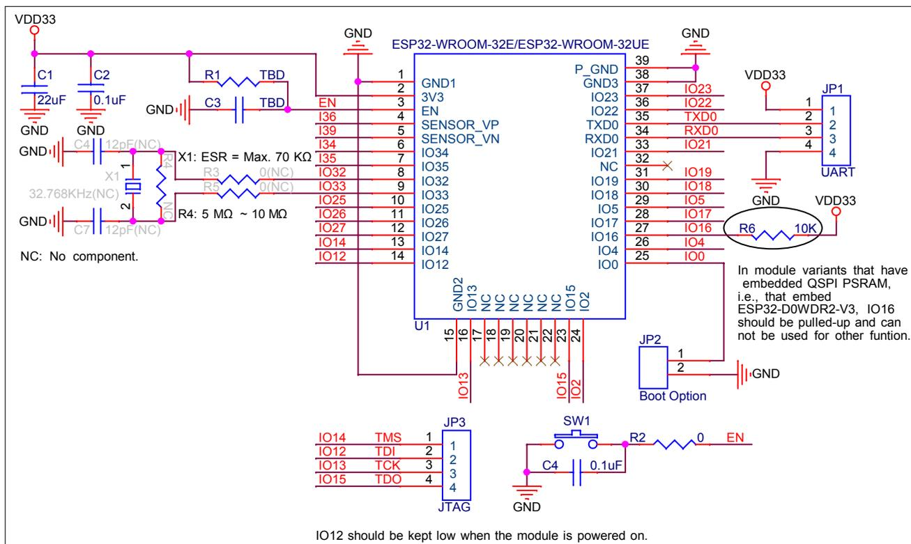
Figure 7: Peripheral Schematics
