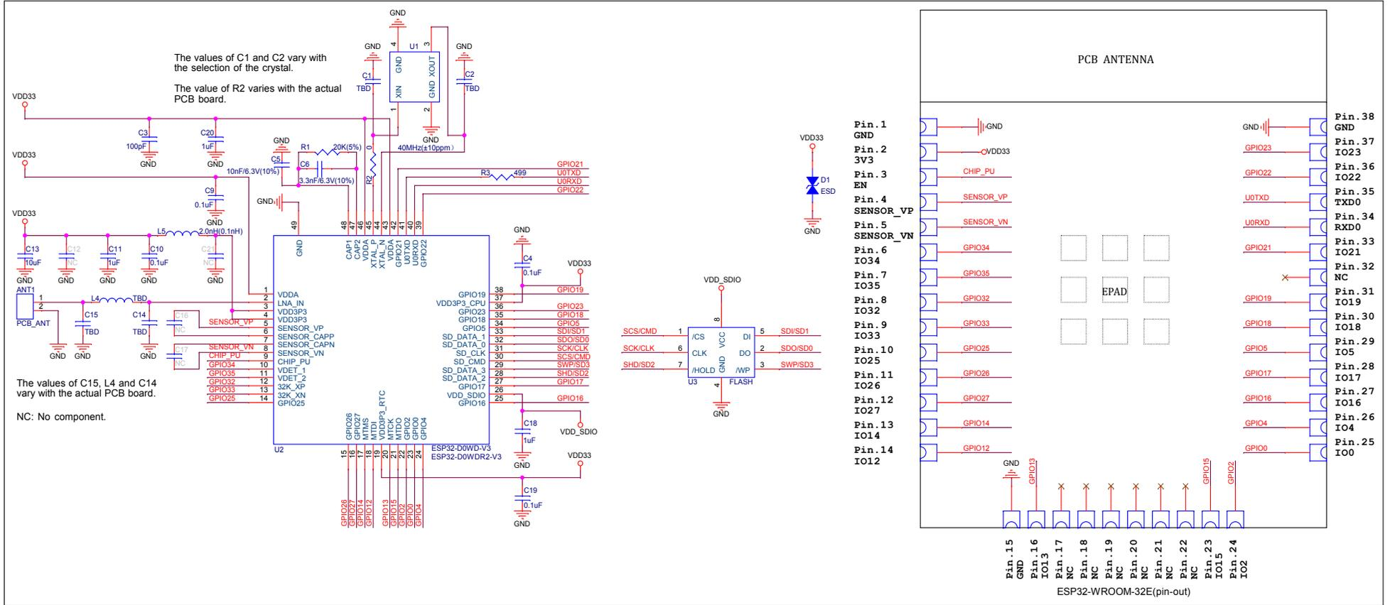
Figure 5: ESP32-WROOM-32E Schematics
