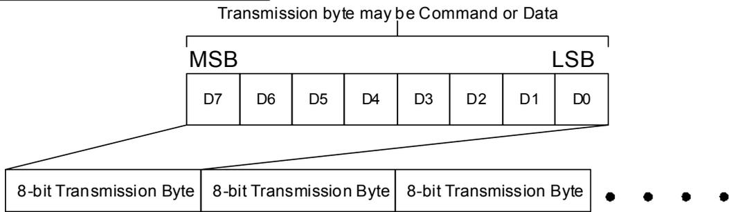
Host processor drives the CSX pin to low and starts by setting the D/CX bit on SDA. The bit is read by ILI9341V on the first rising edge of SCL signal. On the next falling edge of SCL, the MSB data bit (D7) is set on SDA by the host. On the next falling edge of SCL, the next bit (D6) is set on SDA. If the optional D/CX signal is used, a byte is eight read cycle width. The 3/4-line serial interface writes sequence described in the figure as below.
