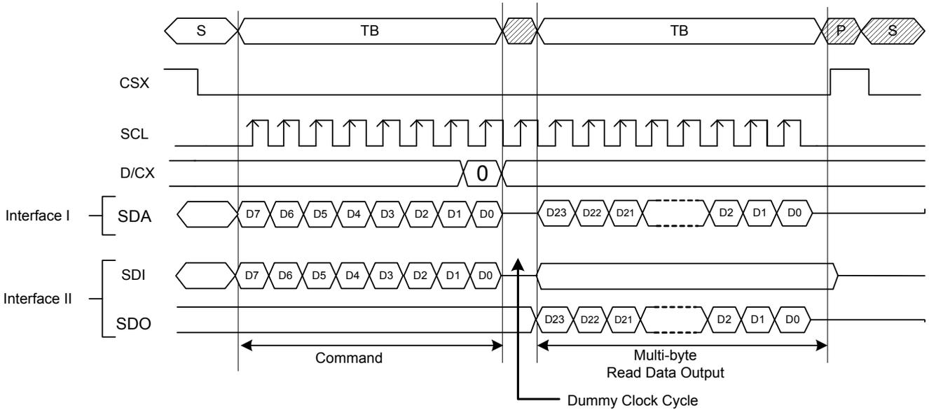
4-wire Serial Protocol (for RDDST command: 32-bit read)
