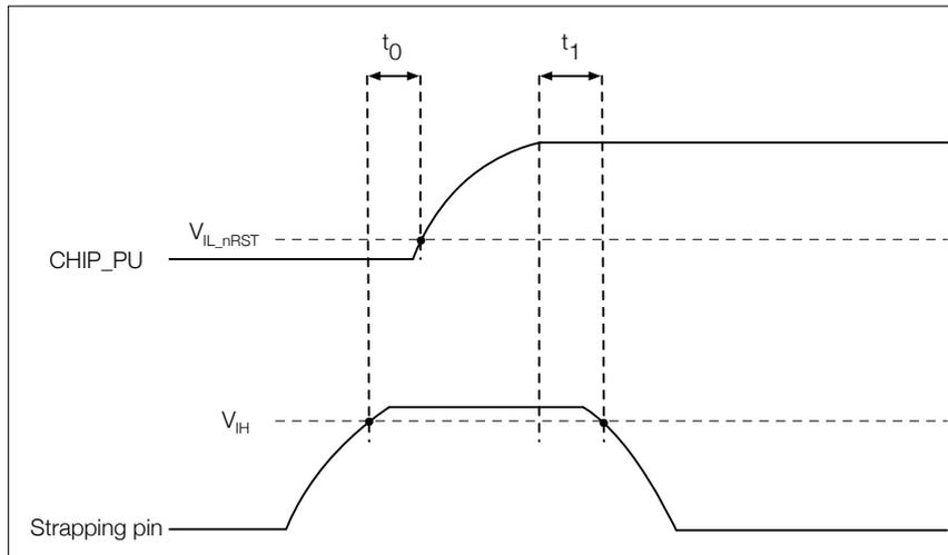
**Figure 4: Setup and Hold Times for the Strapping Pins****Table 5: Parameter Descriptions of Setup and Hold Times for the Strapping Pins**
