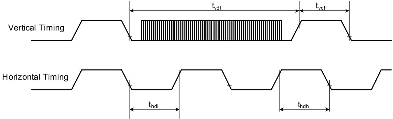
AC characteristics of Tearing Effect Signal (Frame Rate = 60Hz)
