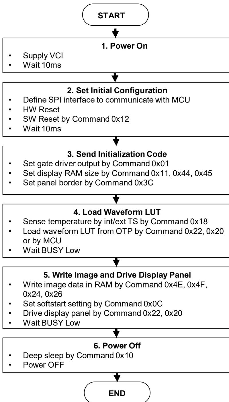
Figure 9-1: Operation flow to drive display panel
