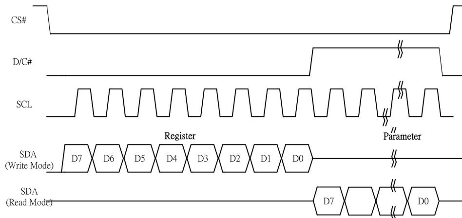
Figure 6-2 : Read procedure in 4-wire SPI mode
