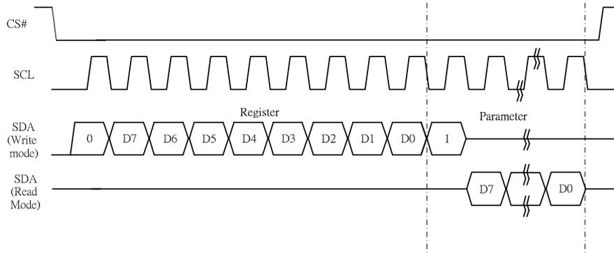
**Figure 6-4 : Read procedure in 3-wire SPI mode**
