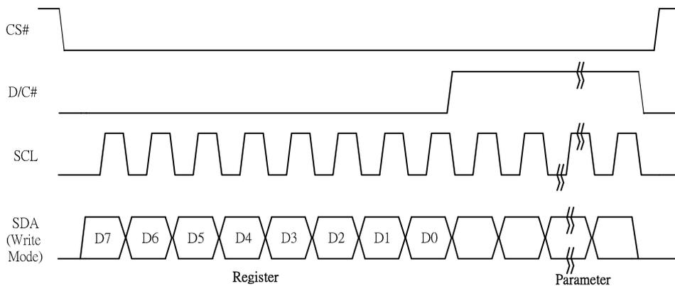
**Figure 6-1 : Write procedure in 4-wire SPI mode**
