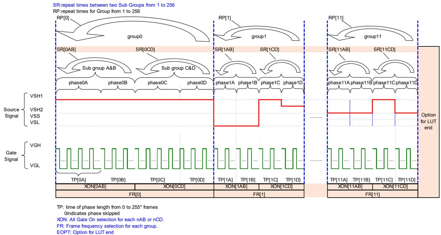
**Figure 6-5 : Gate waveform and Programmable Source and VCOM waveform illustration**
