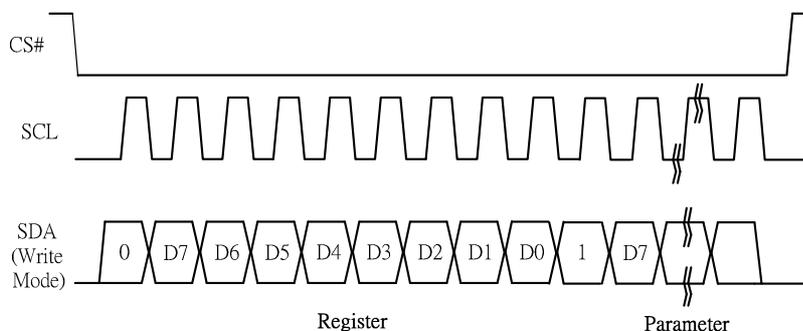
Figure 6-3 : Write procedure in 3-wire SPI
