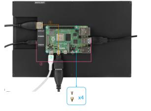
Note: 1.The Raspberry Pi cannot be powered on directly by powering the screen (neither 5V/2A nor 5V/3A). 2. Please connect the cables then power the Raspberry Pi. And use the full 2A for power supply with Raspberry Pi 3B+, 3B, 2B, B+, B+, A, full 3A for Raspberry Pi 4B.
