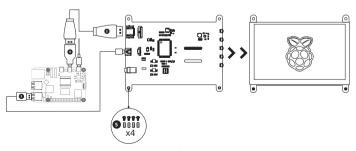
Note: You need to connect the power cable first and then provide power to the Raspberry Pi.
