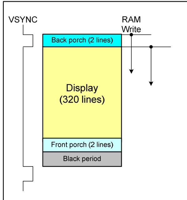
The VSYNC interface has the minimum speed limitation of writing data to the internal GRAM via the system interface, which are calculated from the following formula.
