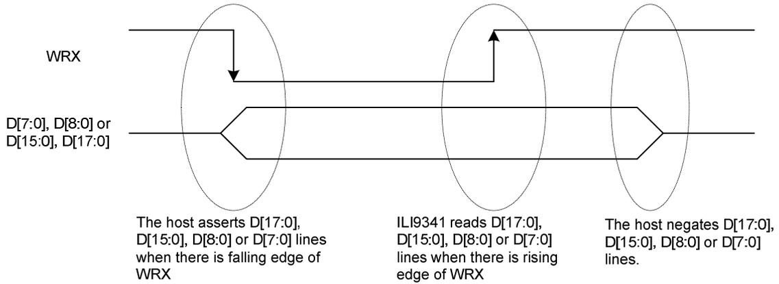
Note: WRX is an unsynchronized signal (It can be stopped)
