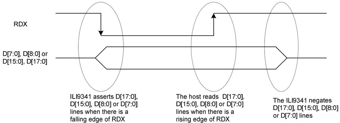
Note: RDX is an unsynchronized signal (It can be stopped).
