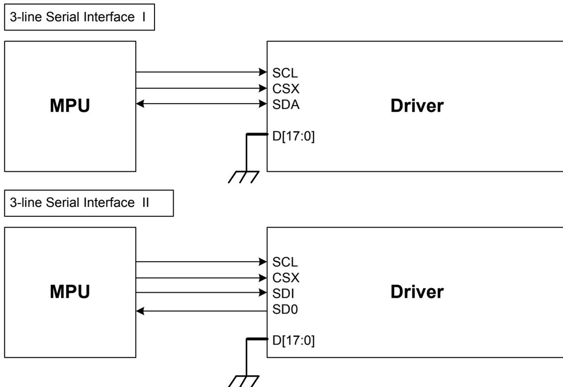
In 3-line serial interface, different display data format is available for two color depths supported by the LCM listed below.
