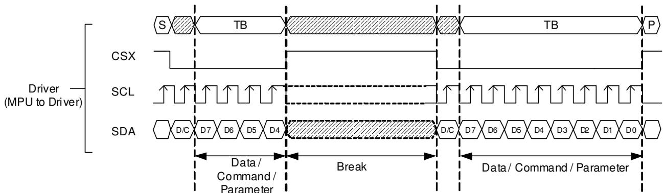
If a two or more parameter command is being sent and a break occurs while sending any parameter before the last one and if the host then sends a new command rather than continue to send the remained parameters that was interrupted, then the parameters which had been successfully sent are stored and the parameter where the break occurred is rejected. The interface is ready to receive next byte as shown below.
