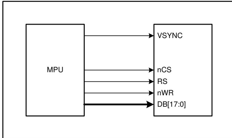
In the VSYNC mode, the display operation is synchronized with the internal clock and VSYNC input and the frame rate is determined by the pulse rate of VSYNC signal. All display data are stored in GRAM to minimize total data transfer required for moving picture display.
