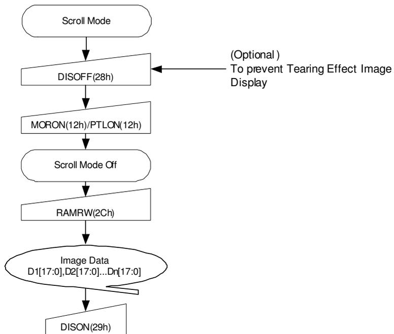
Note: Scroll Mode can be left by both the Normal Display Mode ON (13h) and Partial Mode ON (12h) commands.
