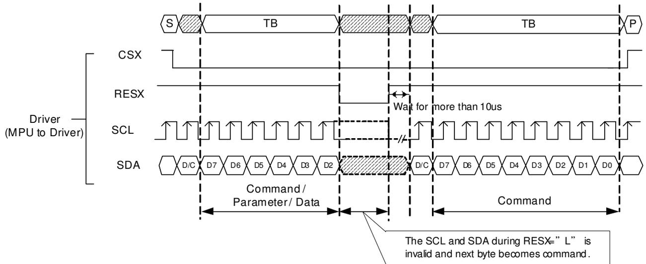
If there is a break in data transmission by CSX pulse, while transferring a command or frame memory data or multiple parameter command data, before Bit D0 of the byte has been completed, then the driver will reject the previous bits and have reset the interface such that it will be ready to receive the same byte re-transmitted when the chip select pin (CSX) is next activated.
