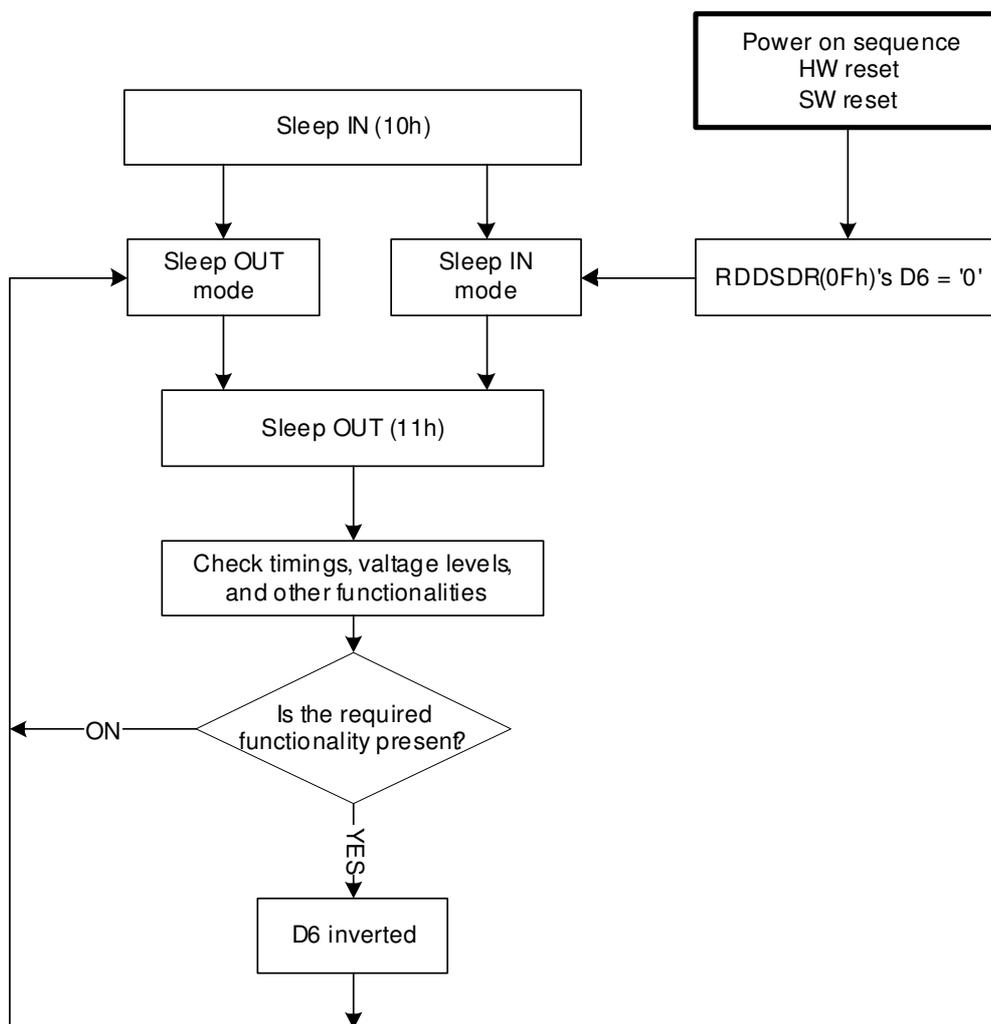
*Note 1: There is needed 120msec after Sleep Out -command, when there is changing from Sleep In -mode to Sleep Out -mode, before there is possible to check if User's functionality requirements are met and a value of RDDSDR's D6 is valid. Otherwise, there is 5msec delay for D6's value, when Sleep Out -command is sent in Sleep Out -mode.*
