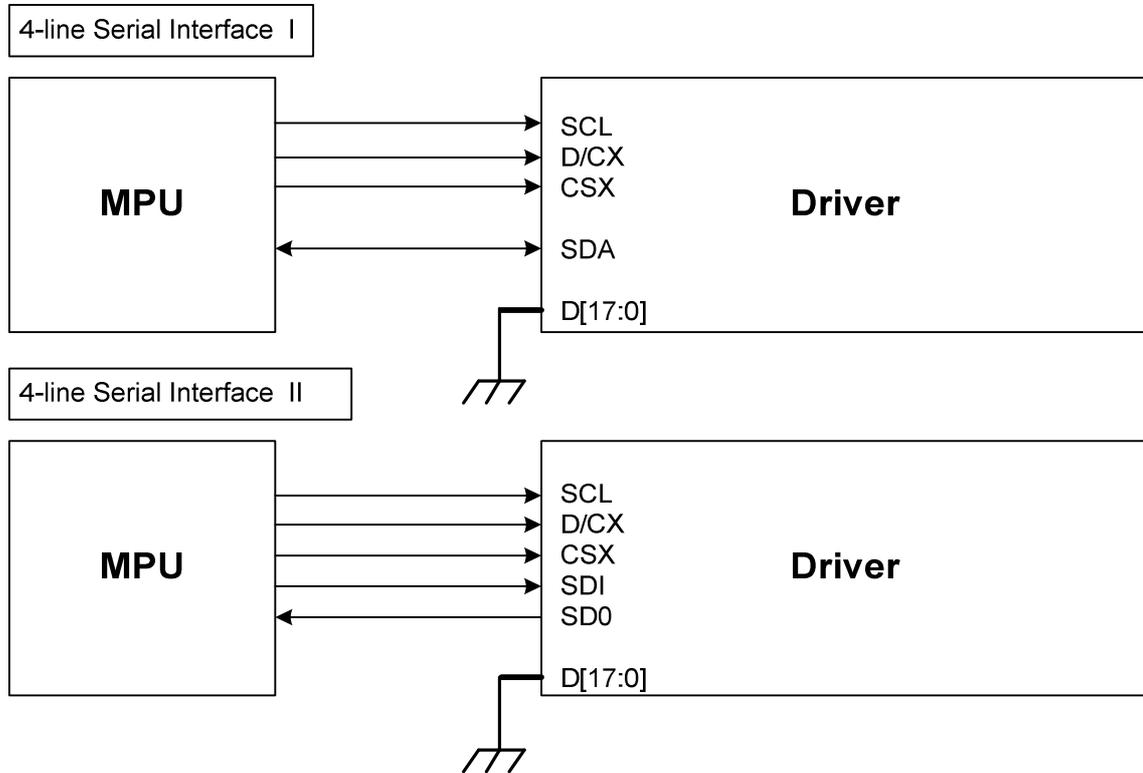
In 4-line serial interface, different display data format is available for two color depths supported by the LCM listed below.
