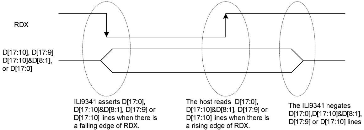
Note: RDX is an unsynchronized signal (It can be stopped).
