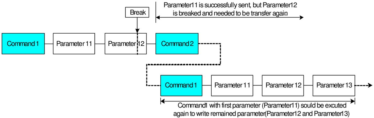
If a two or more parameter command is being sent and a break occurs by the other command before the last one is sent, then the parameters which had been successfully sent are stored and the other parameter of that command remains previous value.
