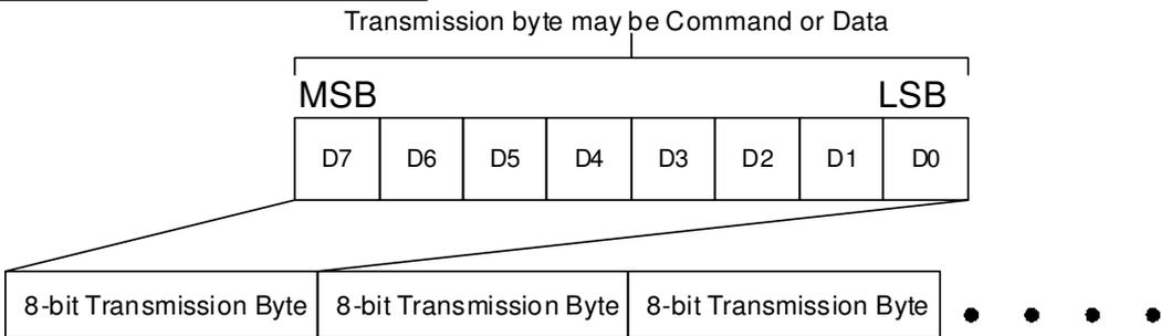
Host processor drives the CSX pin to low and starts by setting the D/CX bit on SDA. The bit is read by ILI9341 on the first rising edge of SCL signal. On the next falling edge of SCL, the MSB data bit (D7) is set on SDA by the host. On the next falling edge of SCL, the next bit (D6) is set on SDA. If the optional D/CX signal is used, a byte is eight read cycle width. The 3/4-line serial interface writes sequence described in the figure as below.
