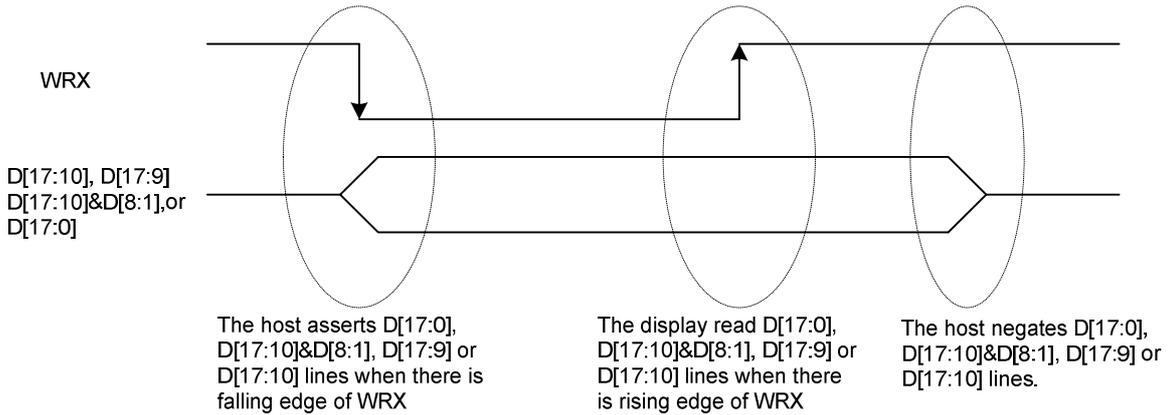
Note: WRX is an unsynchronized signal (It can be stopped)
