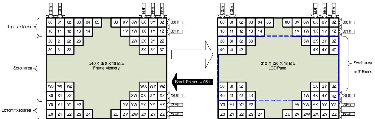
Note: When Vertical Scrolling Definition Parameters (TFA+VSA+BFA) ≠ 320, Scrolling Mode is undefined.
