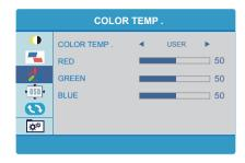
• The color temperature function contains three preset color modes (Cool/Warm/User). When you select the color temperature as Cool/Warm, its corresponding red/green/blue values will also be displayed below. And only under the User Mode, the parameter of RED/GREEN/BLUE could be adjusted by user.
