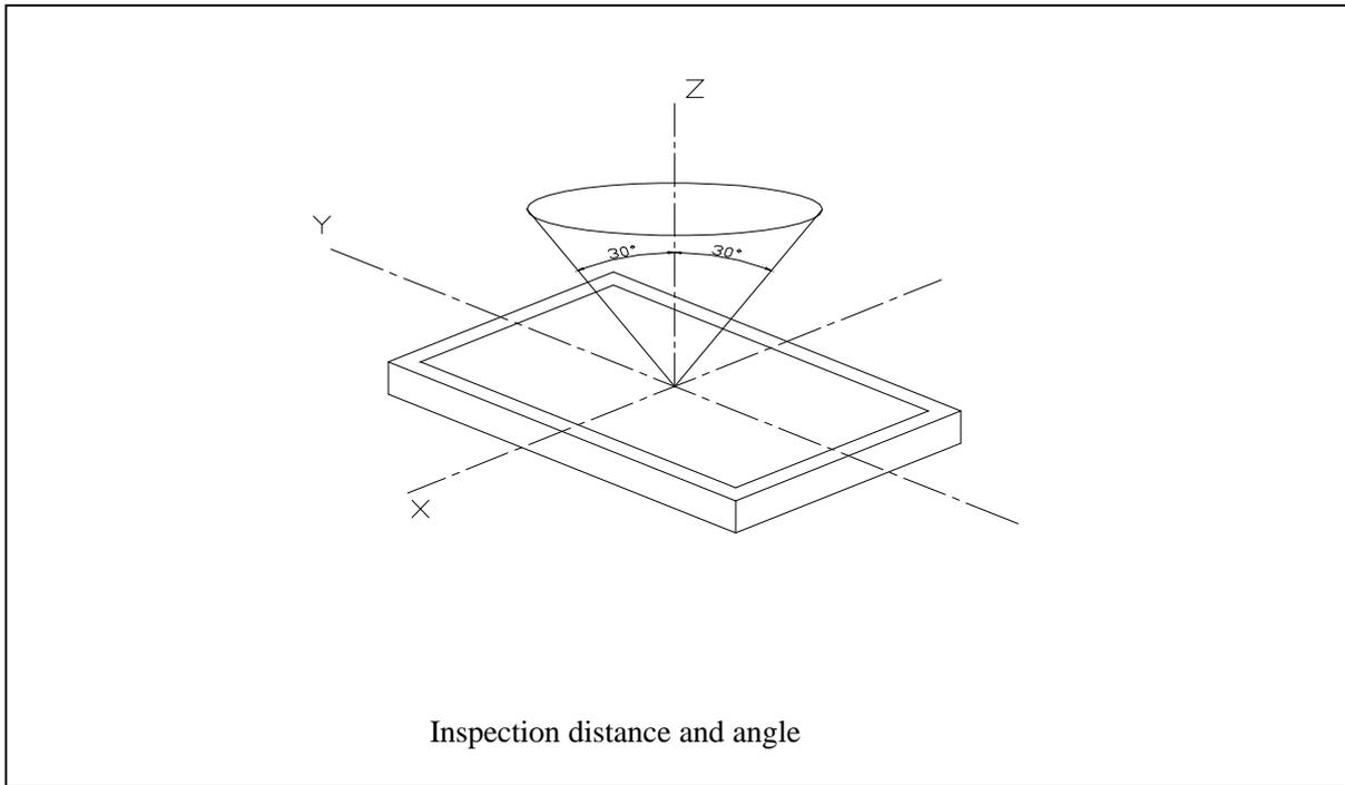
Inspection should be performed within angle  $\phi$  ( $\phi$  is usually  $30^\circ$ ) from Z axis to each X and Y. Inspection distance in any direction within  $\phi$  must be kept  $30 \pm 5$  cm from the display surface.
