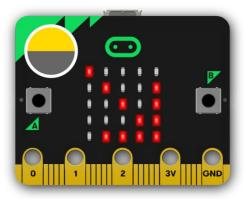
• The temperature sensor transforms the temperature in the ambient environment into digital signals that can be read by the micro:bit for calculating the current temperature of the device.
