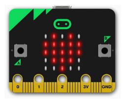
• There are two buttons on the front of the micro:bit - button A and button B, you can detect when these buttons are pressed, allowing you to trigger code on the device. You can detect events such as a single press, a double press, and a long press by programming.
