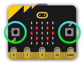
• The LED screen works as a basic light sensor by reversing the LEDs of the screen to become an input, which allows you to detect the ambient light.
