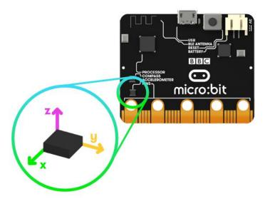
The compass detects the earth's magnetic field, allowing you to detect which direction
