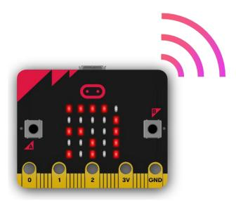
The Bluetooth Low Energy antenna allows micro:bit to send and receive Bluetooth signals, you can wirelessly communicate the micro:bit with phones, PCs and tablets.
