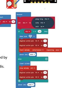
5. If the value of dis more than 10, clear the matrix LEDs, stop melody and turn two LEDs off.6. Loop in forever block.
