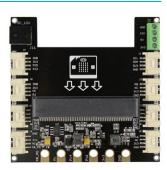
In addition, there is a power port, from which you can draw 3.3V/5V/12V three voltages! This means that when you use a module such as a motor, you no longer need an external drive!
