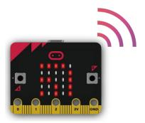
• Bluetooth: The Bluetooth Low Energy antenna allows the micro:bit to send and receive Bluetooth signals, you can wirelessly communicate between micro:bit and phones, PCs, or tablets. You need to pair your micro:bit with another device before using the Bluetooth antenna.
