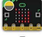
Radio: The radio feature allows you to communicate wirelessly between two or more micro:bits.
