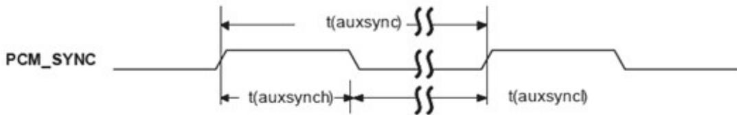
**Figure 225: PCM\_SYNC timing**
