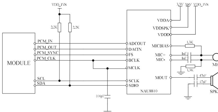
**Figure 258: Audio codec reference circuit**
