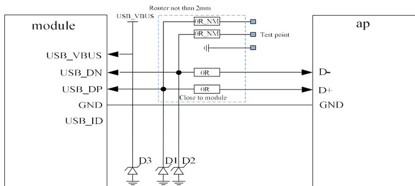
**Figure19: USB reference circuit**
