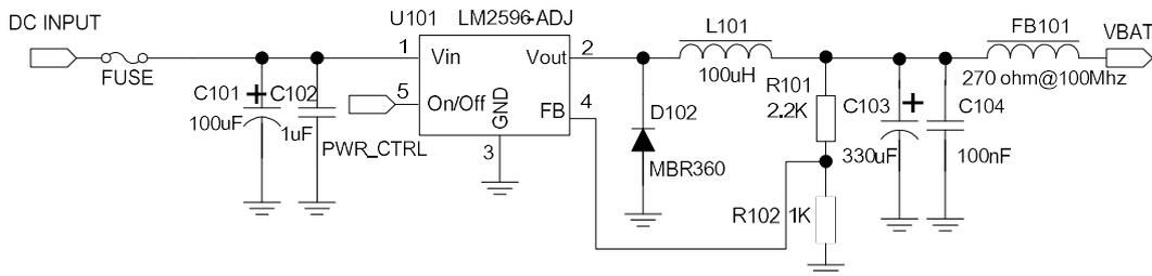
**Figure 8: Switching mode power supply reference circuit**
