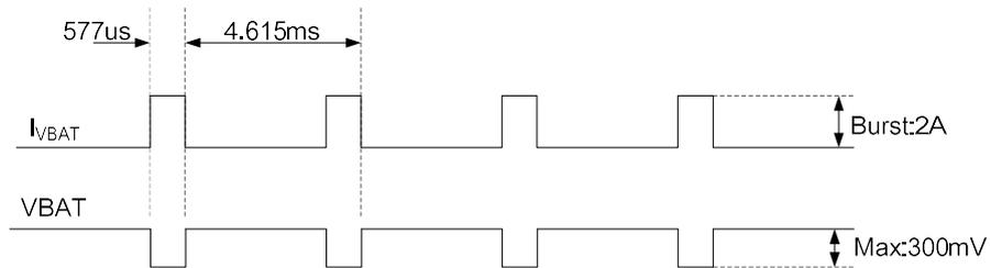
**Figure 5: VBAT voltage drop during burst emission (GSM/GPRS)**
