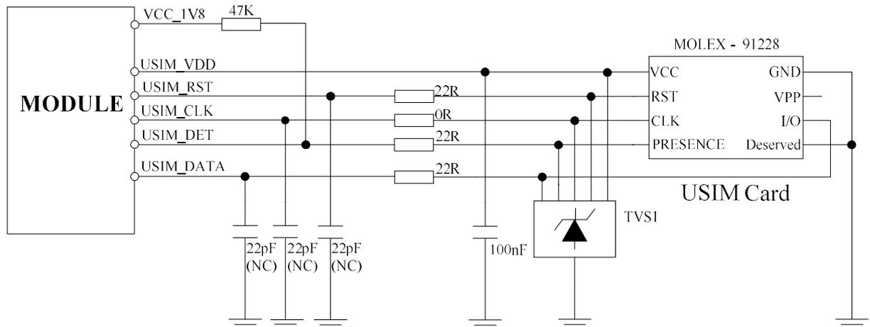
**Figure 203: USIM interface reference circuit with USIM\_DET**
