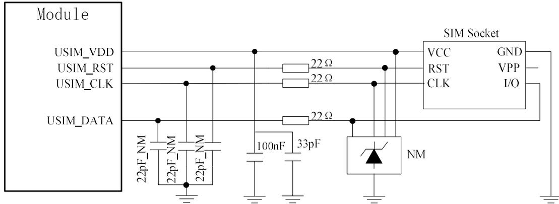
**Figure 192: USIM interface reference circuit**
