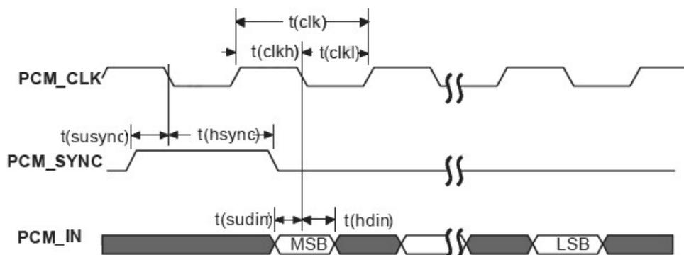
**Figure 236: EXT codec to MODULE timing**
