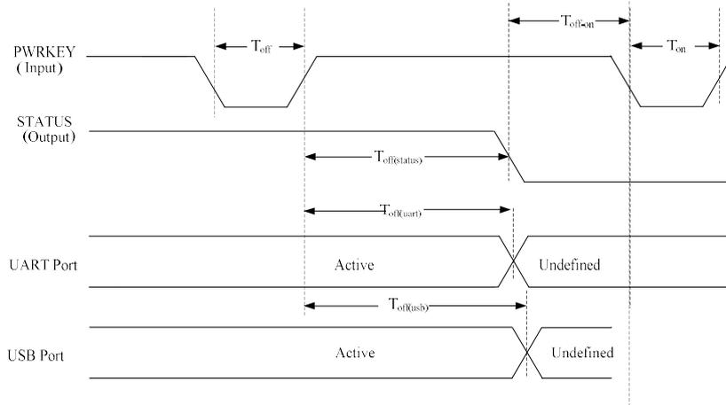
Figure 11: Power off timing sequence
