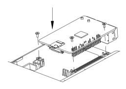
4. Connect the Micro HDMI adapter board to the Micro HDMI interface of the Raspberry Pi.
