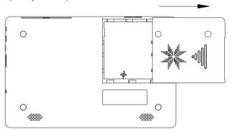
3. Vertically install the Raspberry Pi 4 with the TF card inserted into the Raspberry Pi compartment.
