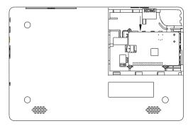
5. Connect the Raspberry Pi power cable and the 2pin interface to the female socket on the PCBA board, and insert the Type-c into the Raspberry Pi type-c power port.
