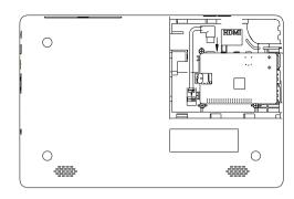
6. Remove the USB head and insert it into the USB port of the Raspberry Pi through the cable hole. It's for camera and microphone.
