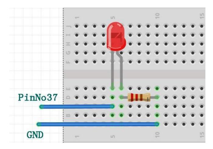
You can refer to this picture to make your circuit on the breadboard. Don't forget that PinNo37 is located on the SERVO1 Interface GPIO port. The GND is located on the SERVO1 Interface as well on the GND port. We'll need to take one resistor that comes with the CrowPi package and wire it to the negative side of the LED (the negative side of the LED is the shorter leg between the 2 LED legs).
