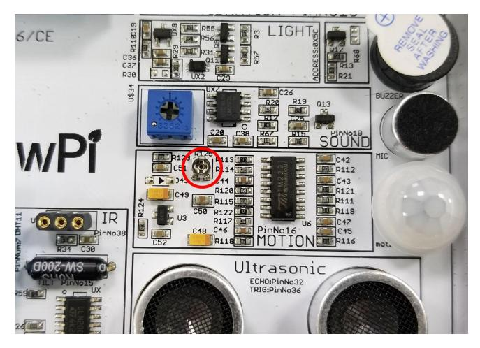
By using a standard Philips flat head screwdriver, rotate the screw to the right or to the left when running the motion example script in order to find a suitable distance for the motion sensor.
