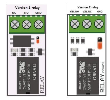
There are two version of Relay in our CrowPi, you can distinguish the version of your CrowPi by the pin name on the relay. Version 1 relay: The names of the three pins on the relay are NO, NC, COM. Version 2 relay: The names of the three pins on the relay are VIN\_NC, VIN\_NO, GND. Note: The method used by different versions of the relay will be different, please choose the method corresponding to your own relay version is to use the relay, otherwise the board may be burned out!
