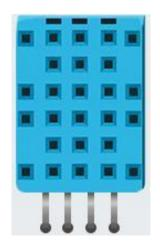
The DH11 is a very interesting and unique sensor as it not only combines one functionality but two! It contains both a humidity sensor and a temperature sensor which are pretty accurate which are great for any weather station project, or if you'd like to check the temperature and humidity in the room and make a smart home project! It can also be used to check the garden humidity and temperature to know if your flowers are in danger or they are cool.
