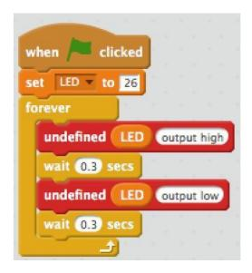
By applying the 0.3 seconds waiting it make the LED turn on and off quickly which makes the blinking effect!
