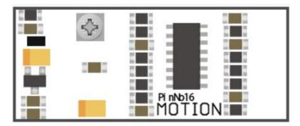
The motion sensor works normally where HIGH means something is moving and LOW means nothing is moving ...
