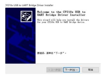
After the installation is complete, connect the USB adapter board in the development kit to the computer, right-click [My Computer], select [Properties], and in the opened [System] interface, select [Device Manager] in the left menu to enter Go to the device manager, expand [Ports], you can see the serial port number corresponding to the recognized CP2102 USB adapter, that is, the driver is installed successfully, and the figure below is COM4.
