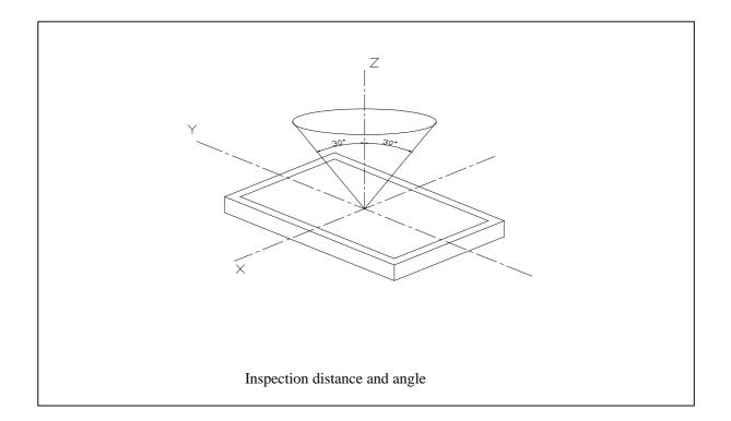
Inspection should be performed within angle $\varphi(\varphi)$  usually 30°) from Z axis to each X and Y. Inspection distance in any direction within  $\varphi$  must be kept 30±5cm from the display surface.
