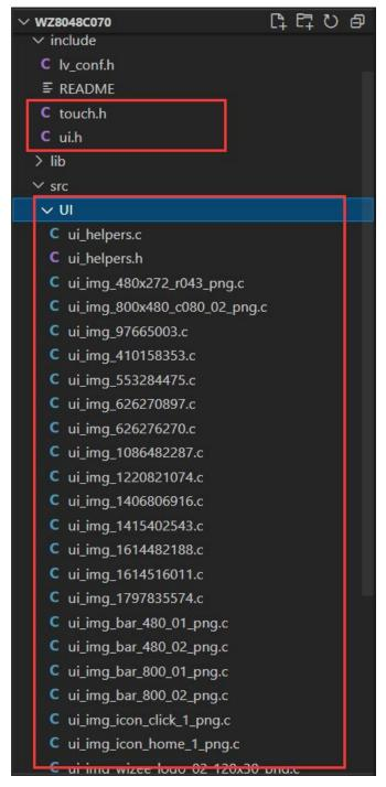
In the UI folder that will be generated. The c file is placed in the /src folder, and in the generated UI folder. Place the h file in the /include folder
