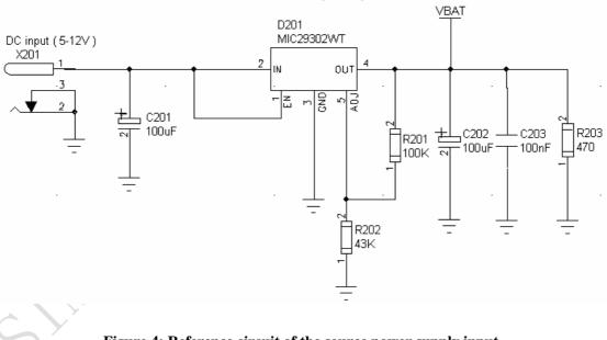
Figure 4: Reference circuit of the source power supply input
