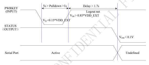
Figure 12: Timing of turn off system using PWRKEY
