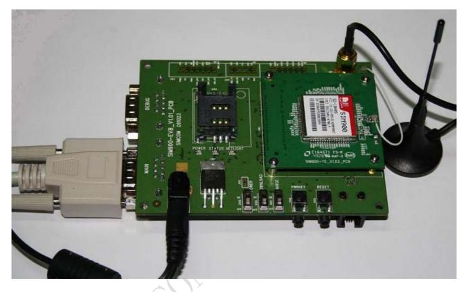
Figure 2: Top view of SIM900 EVB
