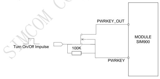
Figure 9: Turn on SIM900 using driving circuit
