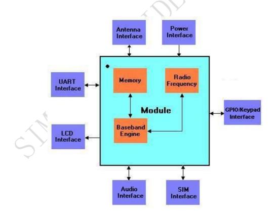
Figure 1: SIM900 functional diagram
