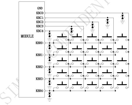
Figure 31: Reference circuit of the keypad interface
