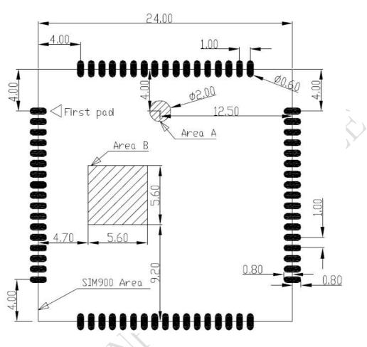
Figure 39: Recommended PCB decal (Unit: mm)
