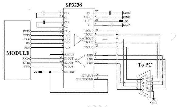
Figure 22: RS232 level converter circuit
