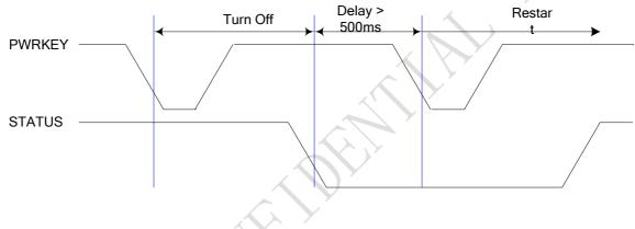
Figure 14: Timing of restart system
