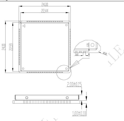
Figure 37: Top an Side Mechanical dimensions of module (Unit: mm)
