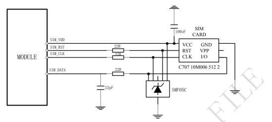
Figure 28: Reference circuit of the 6 pins SIM card
