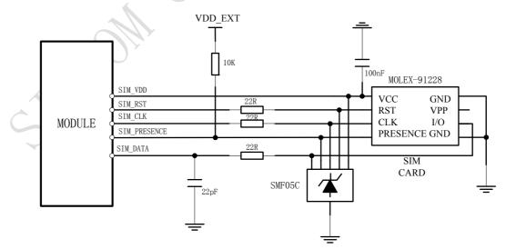
Figure 27: Reference circuit of the 8 pins SIM card
