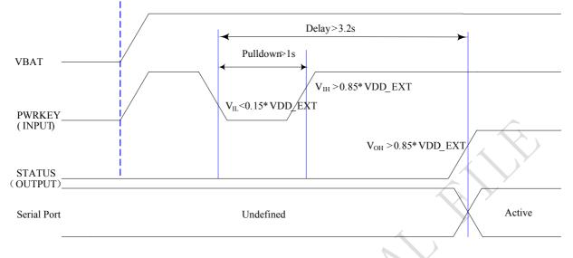
Figure 8: Timing of turn on system using PWRKEY
