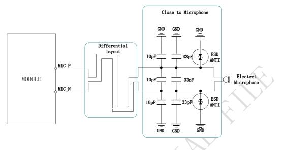
Figure 25: Microphone interface configuration
