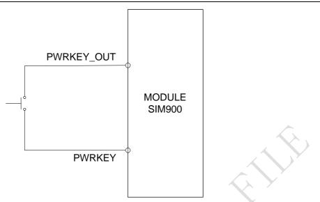
Figure 10: Turn on SIM900 using button
