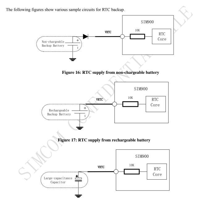
Figure 18: RTC supply from capacitor
